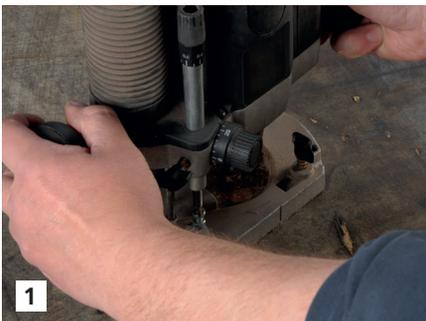
1. Machine out damaged area
