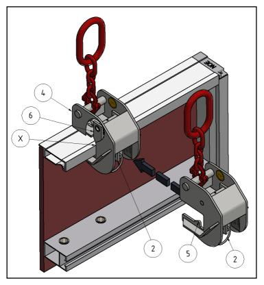
Figure 5: Attaching the Alu-L crane hook
