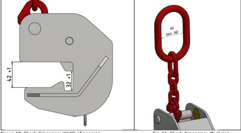
Figure 10: Check dimension: Width of opening
