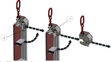
Figure 9: Detaching crane hook
