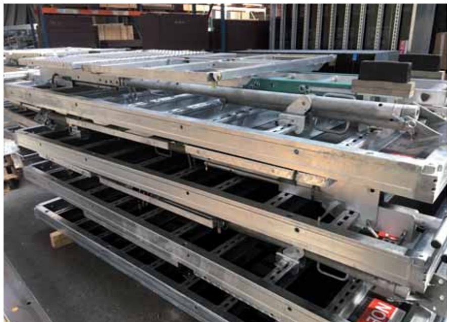
The spacer attached to the back of the NOEtop S panels allows the units to be easily and safely transported.
