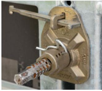
The tapering tie rod can be preset in 10 mm increments using the NOEtop EinsA adjuster nut.
