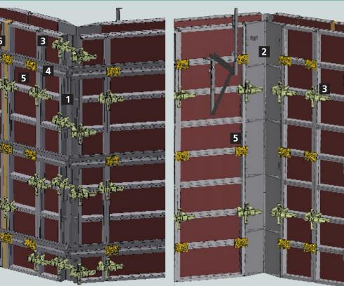
NOEalu L external corner hinge NOEalu L Internal corner hinge 3 NOE Alulock, Part No. 402512 4 Alignment channel, Part No. 135210 6 Compensation piece
