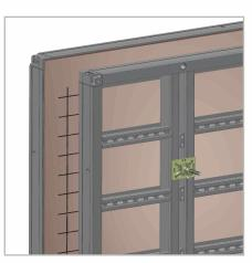
Insert tie rod and install the swivel plate with wing nut
