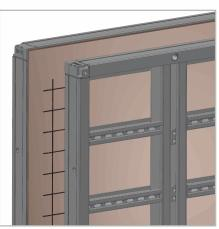
Put second face formwork into place
